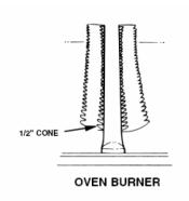
Oven burner flame can be checked as follows (without burner baffle in place):
