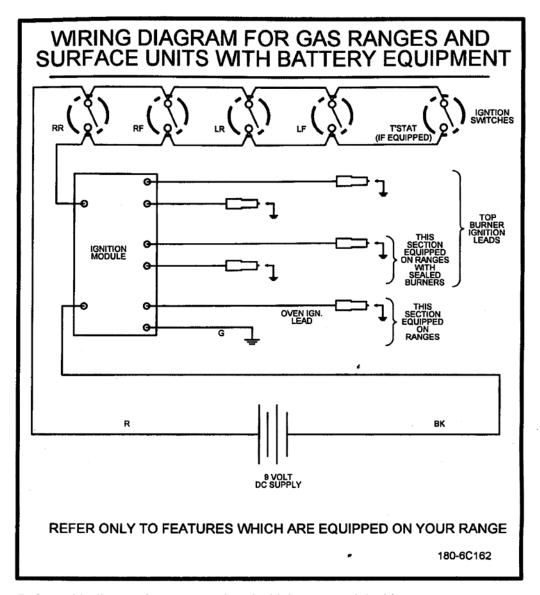
Refer to this diagram for ranges equipped with battery spark ignition.
