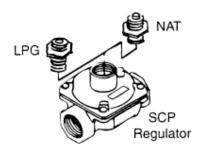
For a Harper-Wyman regulator, remove converter cap by inserting a coin into slot in top and twisting. Turn cap over and re-install.
