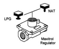
**Note:** What you read on the converter cap or plunger is the type of gas for which the regulator is set. If yours reads NAT, the regulator is set for natural gas. If yours reads LP, the regulator is set for LP.
